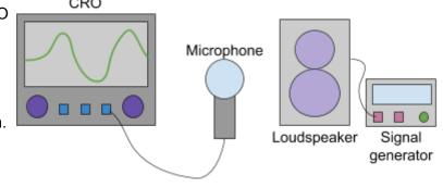
possible, adjust the time-base settings on the oscilloscope.
